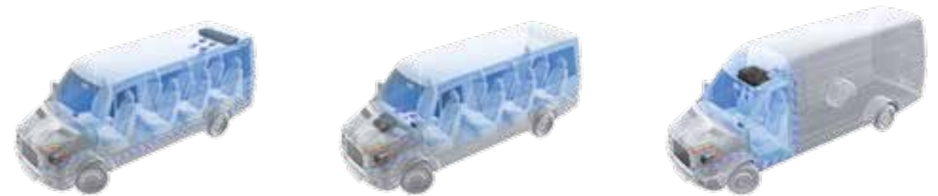
Evaporator under the roof
