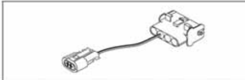
Fig. 2: Test adapter for Thermo 90 S/ST and Thermo 50 MAN/trade heaters, order no. 925 56A
