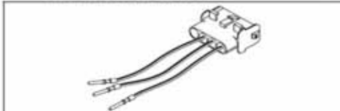
Fig. 3: Test adapter for BBW 46 S and DBW 46 S heaters. You can make an appropriate adapter yourself if required.
